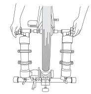
D.2 Tighten and adjust wheel hubtightener on to bicycle rearwheel hub end caps.
