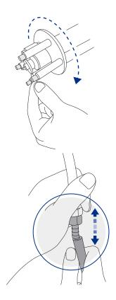
I.3 Open the pump set, remove silicone tube and flip.
