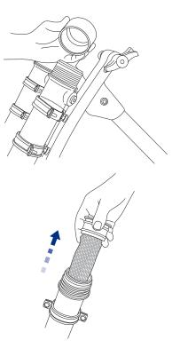
G.2 Remove GoFlow filter slowly and carefully. It might be difficult to remove due to the tight seal.
