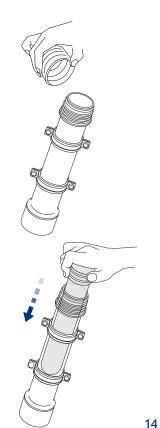
Push filter into housing and ensure H.3 it is flushed to housing.
