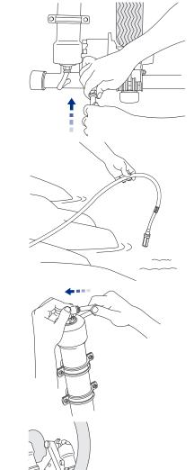
F.2 Post-filter water tube is to be connected to the 2 filter housings using the quick connect fitting. The other end is to be inserted into a vessel to collect the filtered water.
