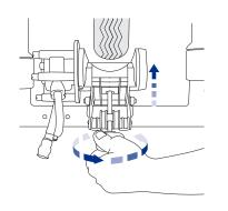
E.2 The bicycle wheel should come into firm contact with the friction roller. When bicycle wheel turns, the friction roller should turn simultaneously.
